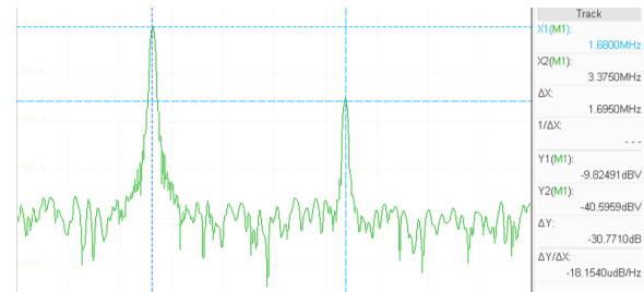
Fig. 9. FFT display at the collector of Q_3 .
